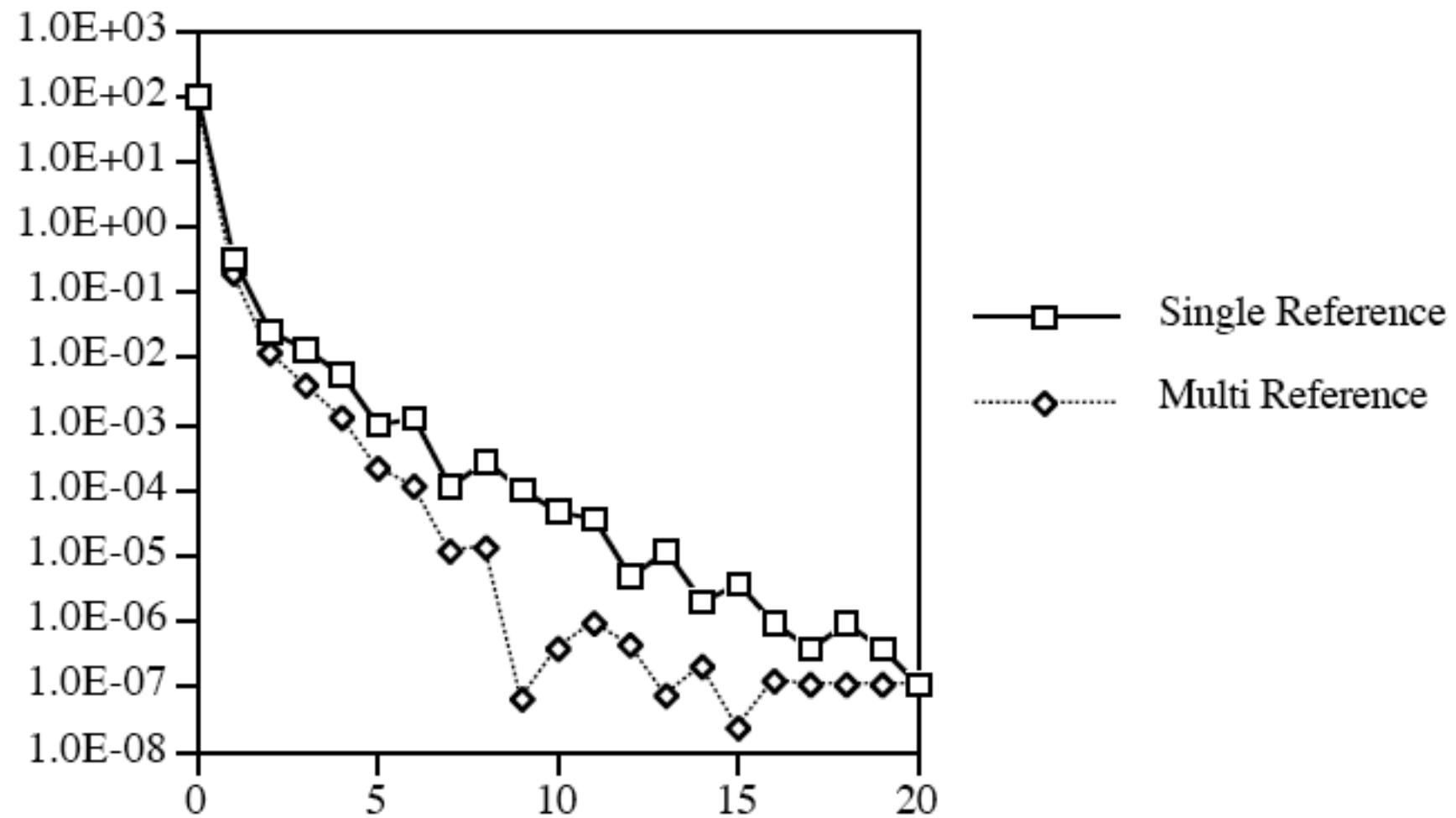
**Figure VI:** Convergence behaviour of the MPPT series of the nitrogen molecule at R<sub>NN</sub> is 5.0 bohr
